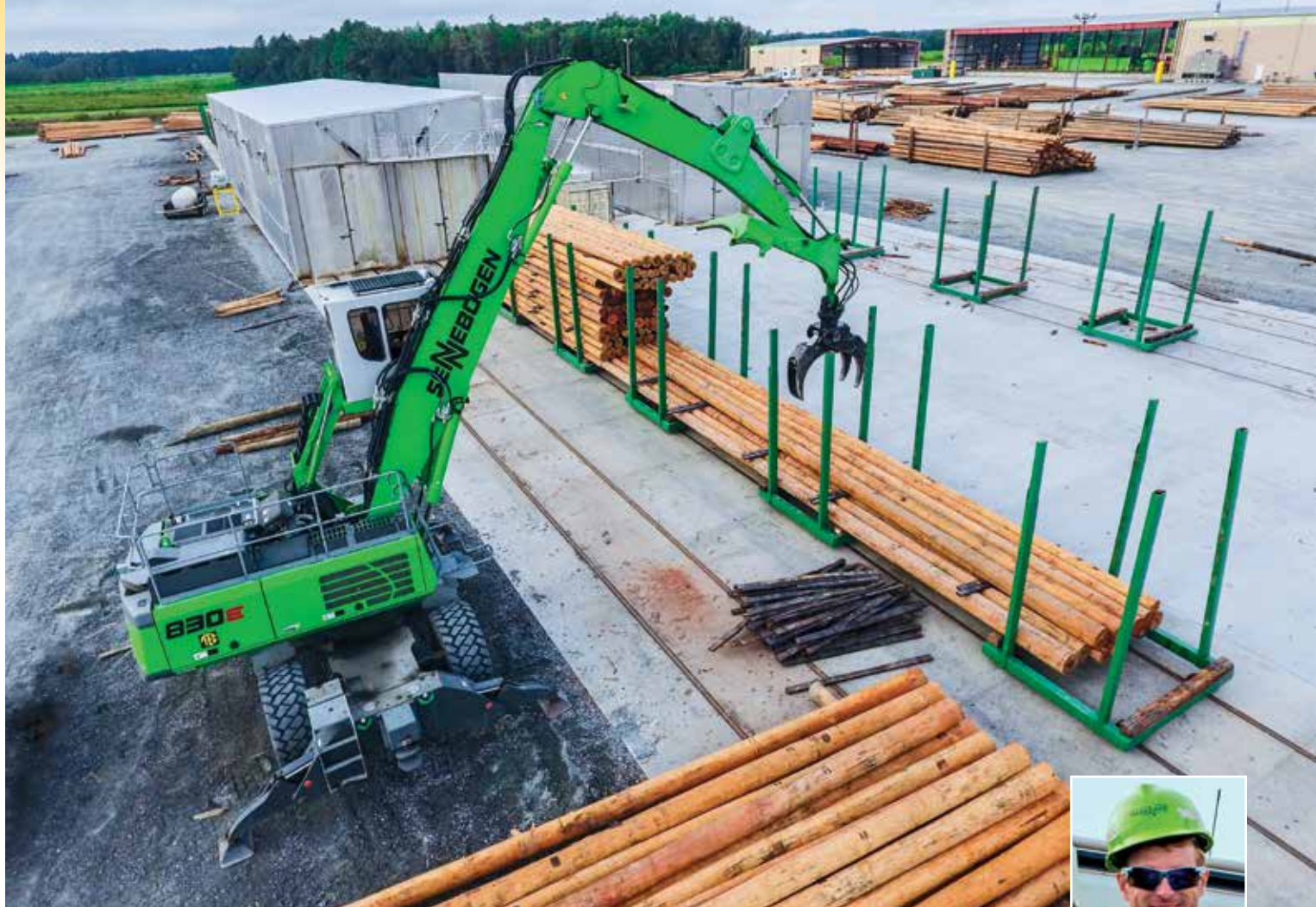
Operator Zachary Singletary uses a SENNEBOGEN 830 E material handler to pick up several poles. "The machine has plenty of reach to lift the poles over the extended arms of the carts quickly and efficiently," noted Singletary. "It's very operator-friendly. The knuckle boom can grab multiple logs, and I don't have to worry about any falling."
