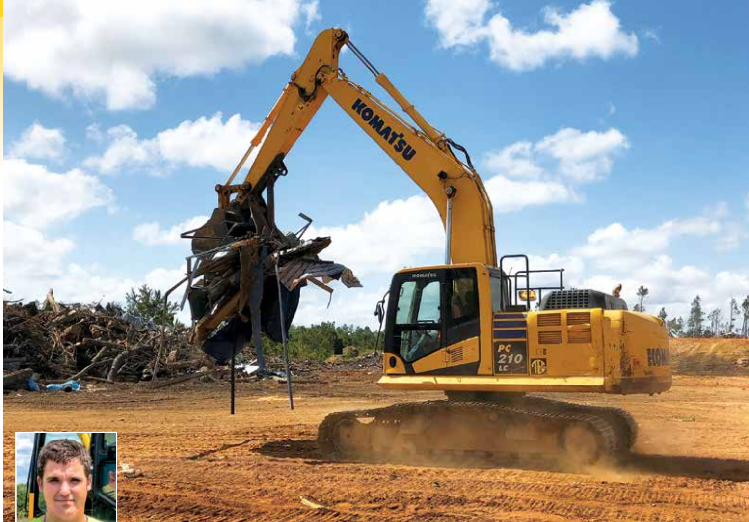
The Komatsu PC210LC excavator is an essential tool for Operator Casey Locke at the Southport, Fla., Waste Pro C&D landfill. He can use the machine to navigate the slope and remove small or large items using the hydraulic thumb attachment.
