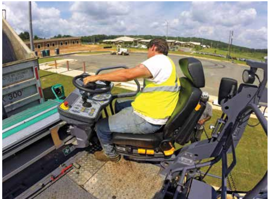
The wide operator platform on the VÖGELE Super 1703-3i wheeled paver provides excellent visibility to the pavement below.
