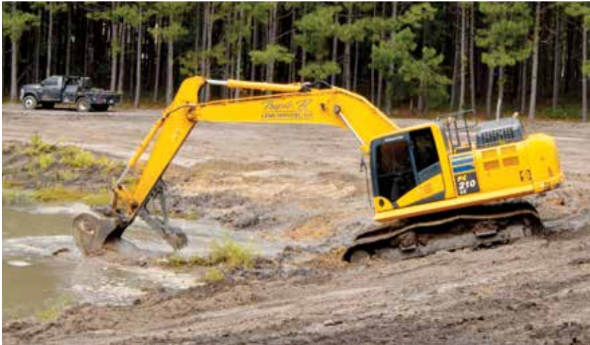
An operator fixes grade at a pond using a Komatsu PC210LC-11 excavator. "We use the 210 in tighter spaces where a bigger machine would get in the way and on mass excavation jobs," said Triple B Land Services owner Ethan Bragg. "From loading dump trucks to knocking down trees, the 210 can handle it. The machine also stands up on the wet areas."
