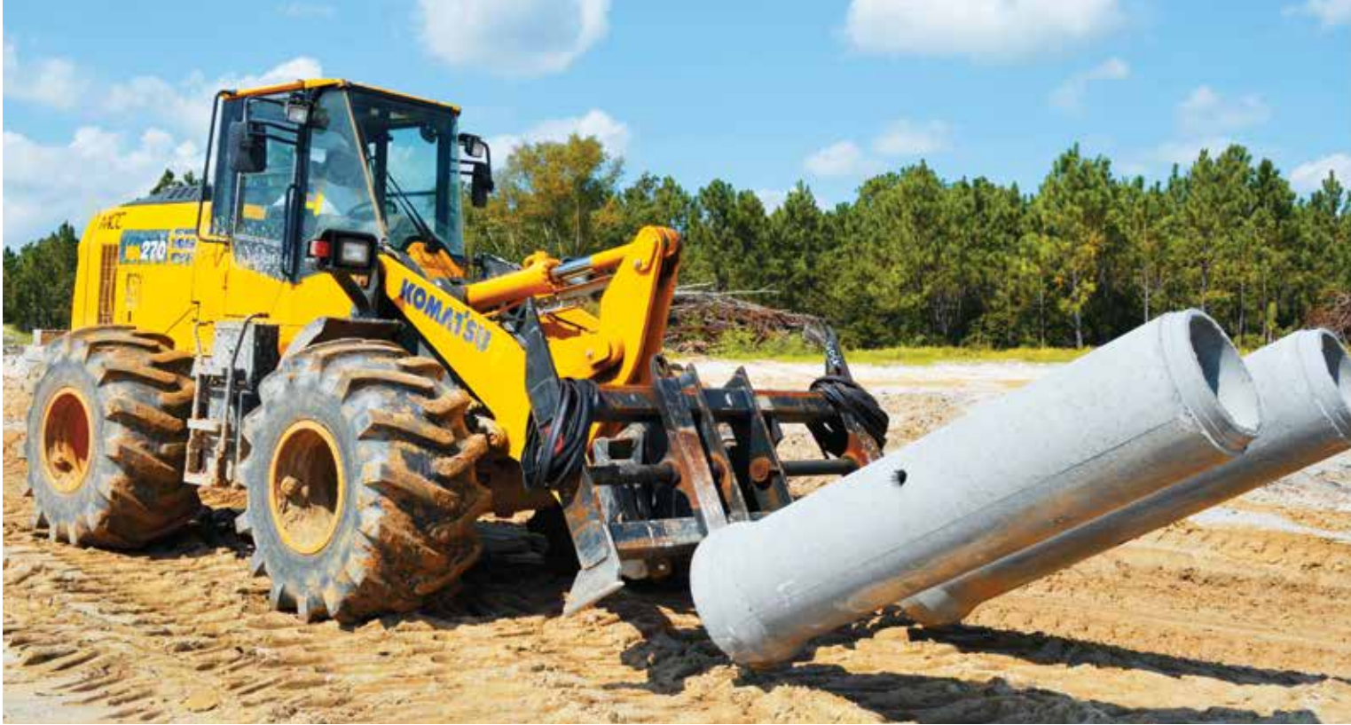
The addition of forestry tires helps a Komatsu WA270 wheel loader work in the sandy and marshy conditions.
