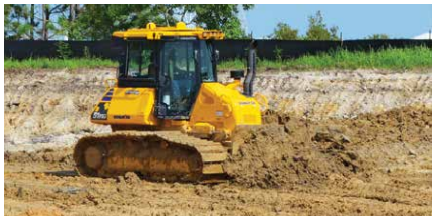
Three Komatsu D51PXi intelligent Machine Control dozers play a big part in the earthmoving accuracy required on the project.
