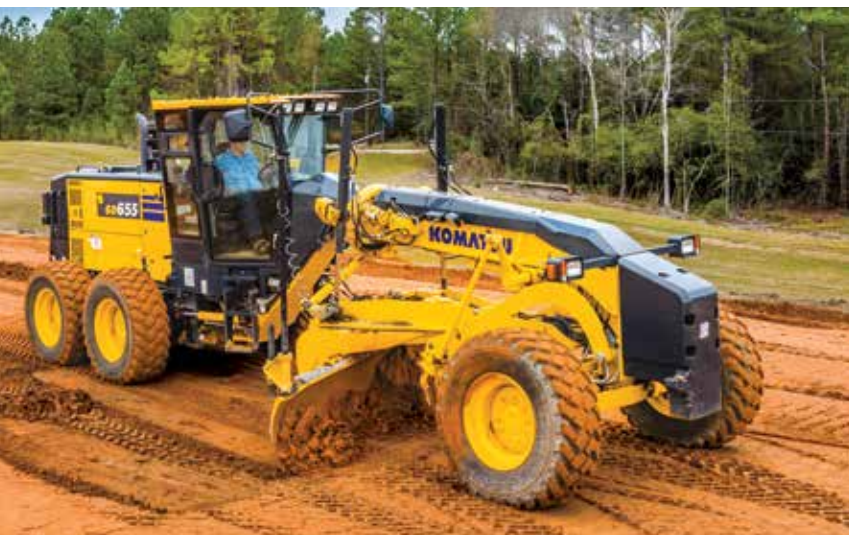
An operator clips a road with a Komatsu GD655 motor grader equipped with Total Station.
