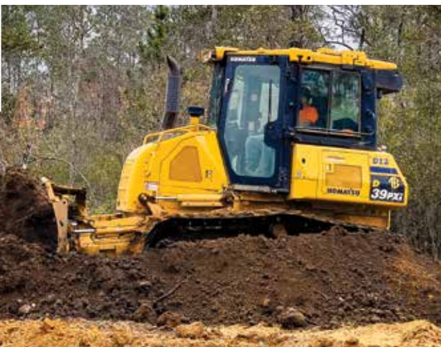
Foreman Dillan Sasser pushes topsoil to grade with a Komatsu D39PXi-24 IMC 2.0 dozer. "It's fairly simple to learn and fun to operate," said Sasser.
